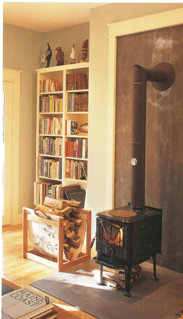
The insulating space of a double-wall stovepipe keeps the smoke hotter as it vents, thus improving the draft, or draw. The tradeoff is that with a double-wall stovepipe less heat radiates into the room.
